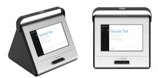
The TUMIGlow Device operates using a touch-screen and utilizes a wi-fi connection to store and share results.
